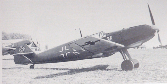
ABOVE: A clear photograph of two Bf 109 E-1s of I./JG 1 (formerly I./JG 131) which appear to be finished in a single upper surface colour. No evidence of a splinter pattern can be determined. Considering the wide variety of camouflage patterns applied to the Bf 109 and the fact that there were many different factories and sub-contractors manufacturing the type it is not beyond the possibility that one or two batches were produced in the one overall upper camouflage colour. It is also unlikely that completion would have been stopped because of a shortage of a specific camouflage colour.
