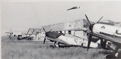
Messerschmitt Bf 109 E-3 Oblt. Werner Pichon-Kalau von Hofe, Technical Officer III./JG 51 Oblt. Werner Pichon-Kalau von Hofe's Bf 109 E-3 as it appeared during the mid-summer of 1940. Finished in a high demarcation 70/71 camouflage scheme it carried the III.Gruppe 'Axt von Niederrhein' beneath the cockpit ledge.
