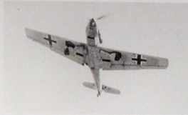
ABOVE: Bf 109 E-1 'Black 12' of 1/JG 27 is pictured here shortly after taking off for a mission during the summer of 1940, showing to good advantage the uneven cycling of the undercarriage as it is retracted. Note also that the flaps are still in the partially lowered position to assist in taking off.
