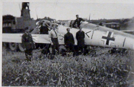
ABOVE AND ABOVE RIGHT: In these two photographs, Oblt Werner Bartels' Bf 109 E-1 has now been raised and had its undercarriage extended in preparation for removal from the site of its forced landing.
