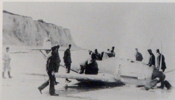
ABOVE, ABOVE RIGHT AND RIGHT: A common occurrence, due to the lack of endurance, was that many Bf 109s ran short of fuel and barely made it back to France or had to ditch in the sea. Here another Bf 109 E-4 of JG 51 has made a belly landing on a French beach during a receding tide. German Luftwaffe personnel are trying to salvage the aircraft before the water returns.
