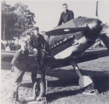
A clear photograph of the nose and cowling of a Bf 109 E-1 showing the original low demarcation colour of RLM 70/71 over 65 camouflage finish.
