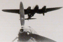
LEFT AND BELOW: Two photographs showing a visiting He 111 landing at JG 2's airfield at Otterville in early August 1940. Of note on the JG 2 Bf 109 in the foreground, is the heavily applied 'stipple' mottling over the RLM 65 on the fuselage side and the motor car type rear view mirror mounted on the canopy framework.
