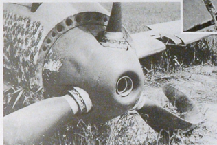
AUGHT AND BELOW: A closeup view of the cockpit and spinner areas of a force-landed Bf 109 E-3 of JG 2 clearly showing the heavily applied green (RLM 70) brush or sponge stipple that was beginning to be applied by the ground crews of this unit at this time. The aircraft was damaged by machine gun bullets which penetrated the engine and cockpit side panels. The broken plexi-glass shows how thin and vulnerable the material was which led to an additional armoured glass panel being applied to the front windscreens on many aircraft. Note part of the JG 2 'Richthofen Geschwader' badge below the cockpit which has been crudely stippled around.
