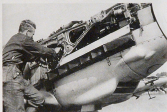
BELOW: A mechanic carries out maintenance to the Daimler-Benz DB 601 engine on a BF 109 E-3 somewhere in France during 1940.
